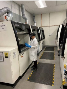
Technician inspects AddiFab 3D-printed mold at MCAM’s Innovation and Technology Center in Arizona
